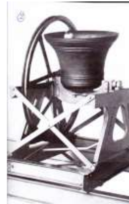
A bell is able to be set in an upwards position when a wooden stay (shown pointing upwards in the picture on the left) rests against a slider at the bottom of the frame
