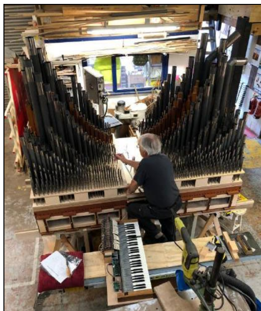
The Great flue ranks of St Peter's, Wolverhampton Willis organ being set up and regulated in Michael Farley's workshop
